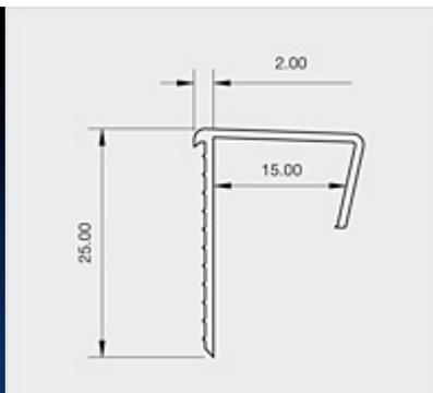
Locally manufactured from recycled plastic, Renderplas PVCu clip on edge beads / board stops are designed for plasterboard and cement board to provide protection to edges and a superior finish. On plasterboard at edges formed at door frames, windows and skirting boards or at a change of finish; on cement board at the exposed edge of the system
